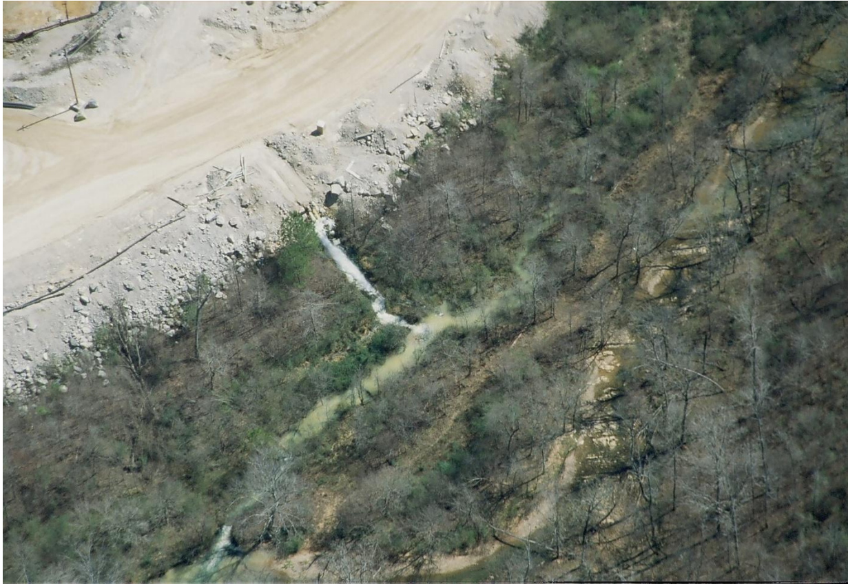
Figure 12. Aerial photograph taken by N. Brooke on 10 May 2004 showing outfall from Bessemer Quarry with heavy siltation and turbidity. The natural flow of Fivemile Creek, seen to the right in this image, is barely visible in comparison to the pale and sediment-laden effluent.
