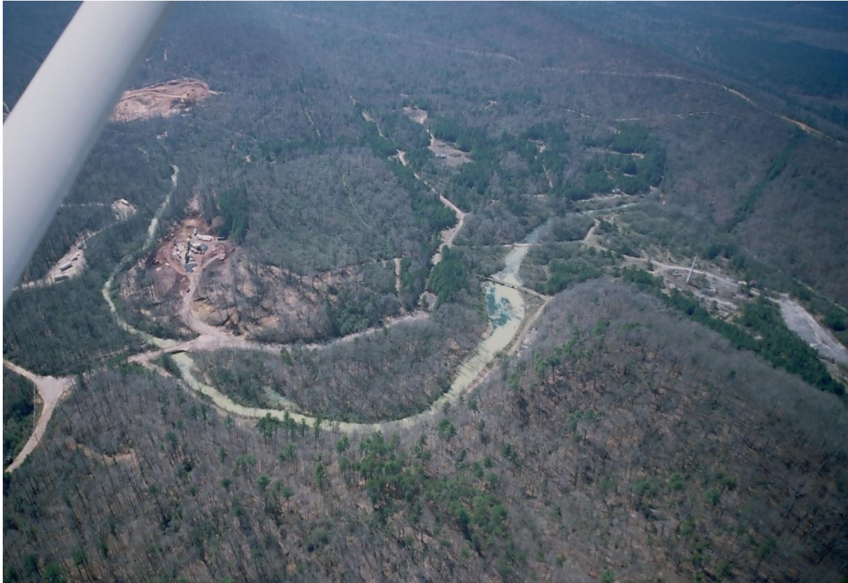
Figure 13. Significant downstream turbidity in Fivemile Creek due to outflow from Bessemer Quarry. Photo taken on 10 May 2004 by N. Brooke.
