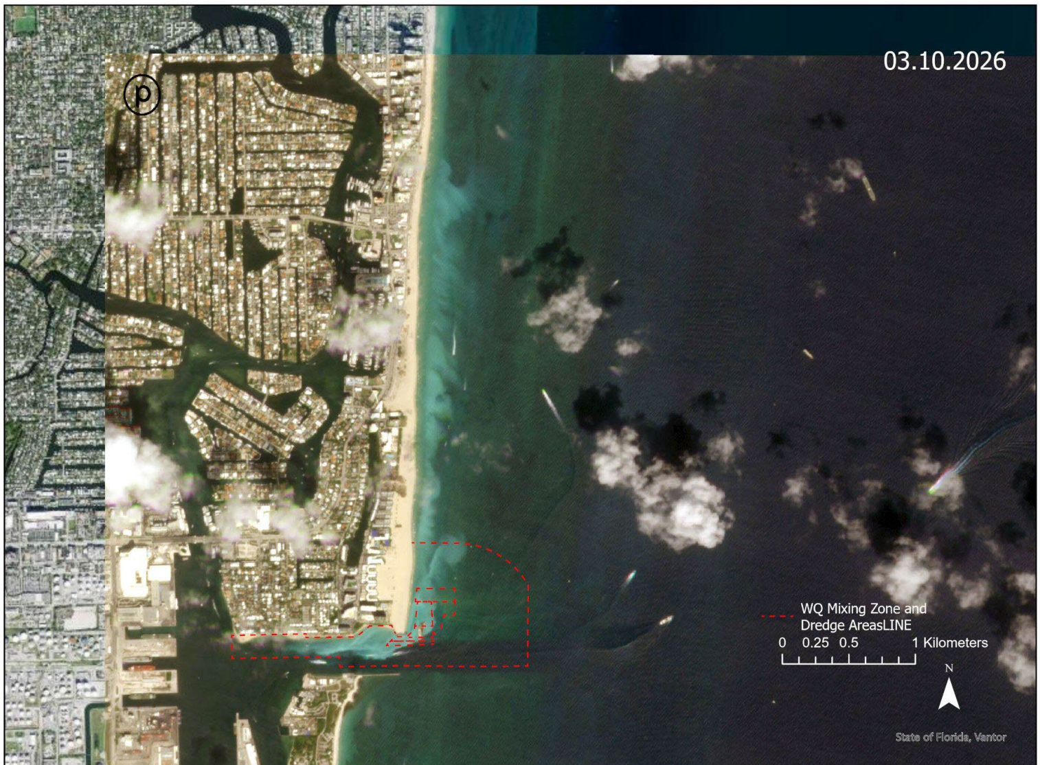
Figure 7A. Satellite showing extent of sediment plume relative to the Sand Bypass project initial construction mixing zone, taken on March 10, 2026 at 11:42 am ET. Imagery is derived from SuperDove true-color data. The approximate distance from the northern edge of the mixing zone boundary to the visible northern edge of the plume is greater than 2,500 meters.
